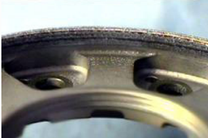
Examples of superalloy components repaired with the LENS process.
