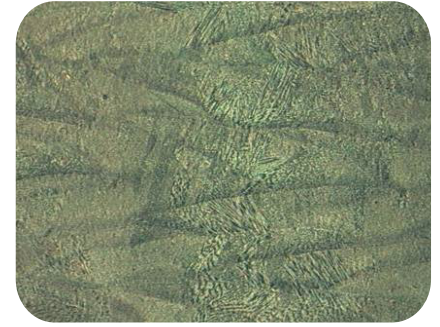
Macrostructure of LENS-deposited IN718, showing elongated grains in the Z-direction, and horizontal curved bands that indicate the layers of the build.
